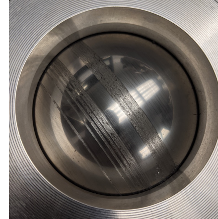
Protected (L) and directly exposed (R) valves tested with highlands simulant and experiencing galling failure at <300 cycles.
