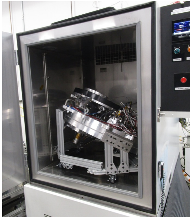
Operation of mechanisms at -45^{\circ}\text{C} (Regolith supply hopper removed)
