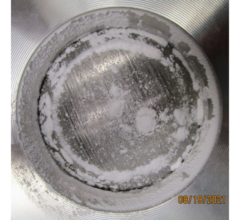
Protected (L) and directly exposed (R) valves tested with highlands simulant and experiencing galling failure at <300 cycles.
