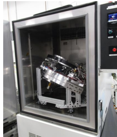
Fig. 4 Carbothermal reactor in a thermal chamber demonstrating operation at expected lunar temperatures.
